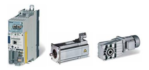
The 8400 HighLine stands out from the 8400 range with its integrated point-to-point positioning. This allows up to 15 selectable target positions, including their travel profiles, to be saved in the inverter. Depending on accuracy and dynamic requirements, you can choose to position with or without feedback.
